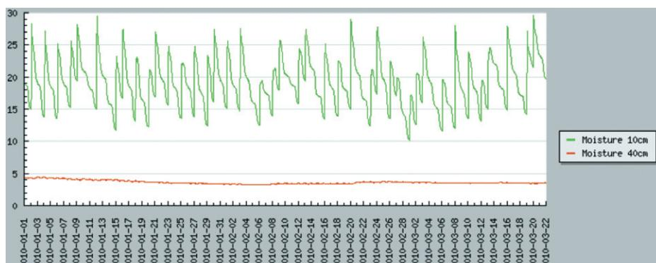
**The sensor-controlled irrigation scheduling resulted in minimal amounts of water getting down the sand profile to 40cm (no leaching losses).**
