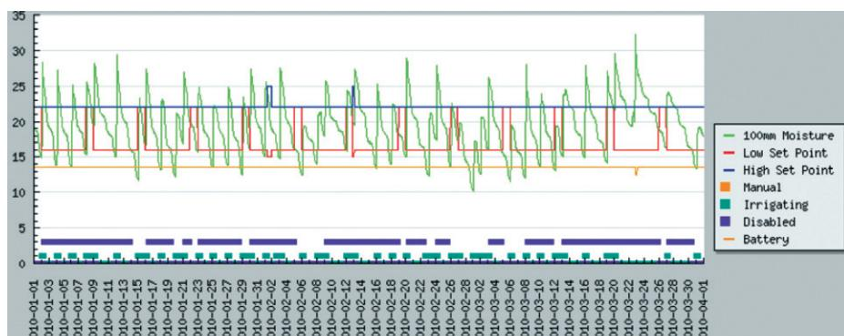
**In effect, the soil moisture in the top 10cm of the turf root zone oscillates between just above the “high” set point and just below the “low” set point.**
